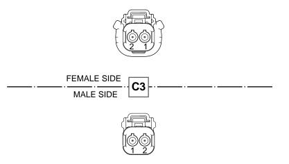
Figure 8. Choke Solenoid Connector Pin Number Identification
